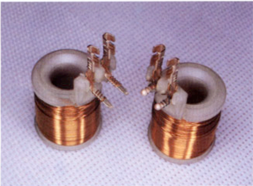
fig.9C. Today's automotive electronic fuel management and antiskid brake systems request highest reliability for components, like coils, responsible for safe and reliable operation of the system. The coil winding ends of the magnet wires are welded with the <spirflame> to the terminal spade. The heat transfer is quick and a minimum of heat energy is induced into the terminal material. The terminal fixed in the plastic mould does not soften by its low temperature the strength of embedding.
