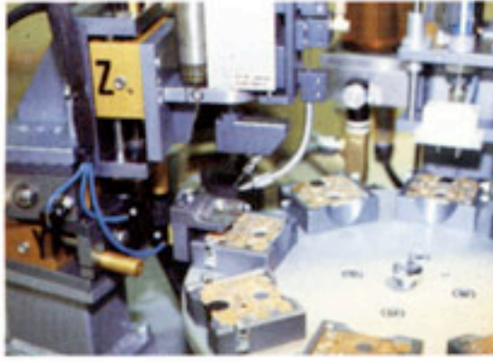
fig.3A. Automated microflame soft soldering on printed circuit boards is an established application.
