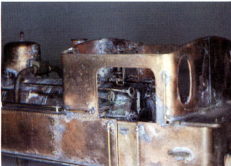
fig.13C / 13D. Manufacture of custom designed down scaled models of locomotives and other carts demands patience and an enormous skilled craftsman to join the many small parts made from thin brass or copper alloy sheet metal.
