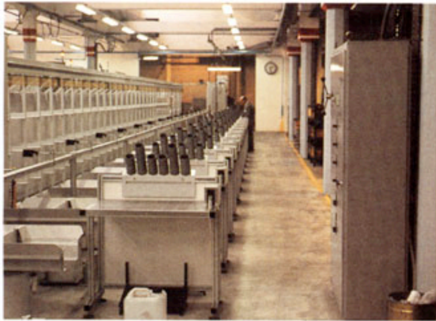
fig.10A. Twenty-one manual operated welding stations are served by 2 banks of each 4 piece model 205HP SPIRFLAME ® s conveniently located at both ends of the group of operator stations.
