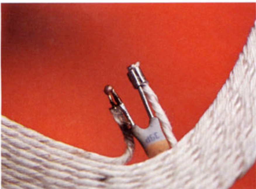
fig.9E. The coil wire ends and capacitor lead ends are welded together in a smooth ball joint.
