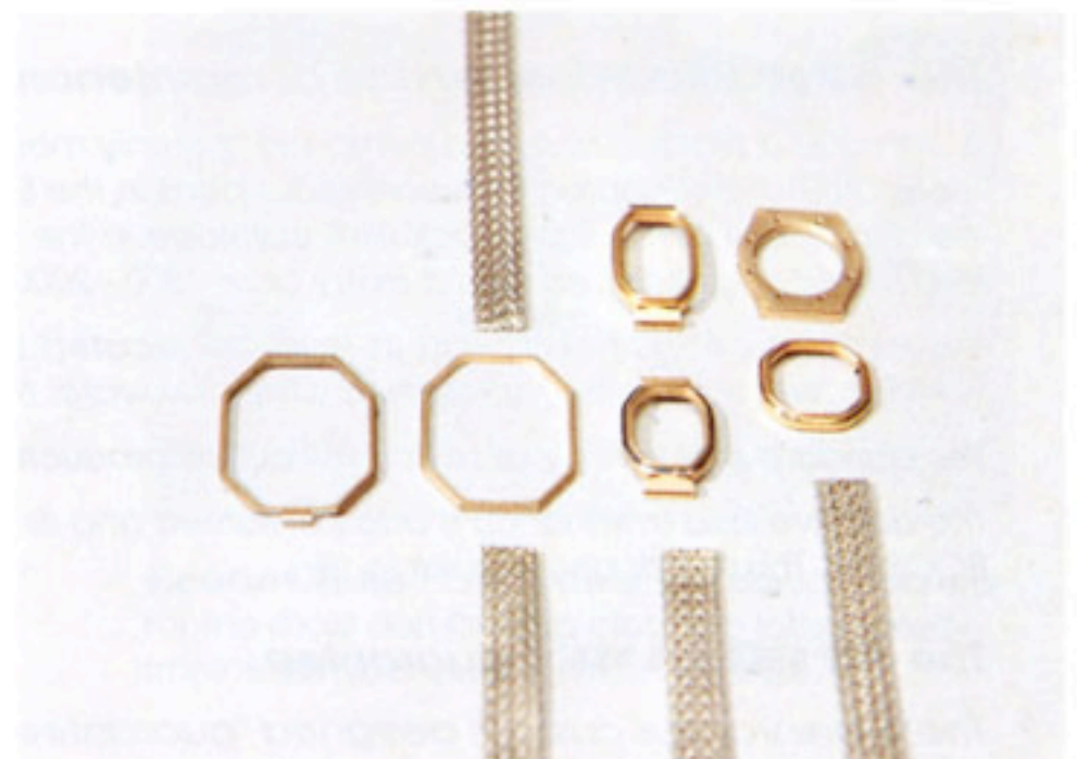
fig.13E. Almost all Swiss manufacturers of jewelry watches use the <spirflame> to gold solder watchcases to the wriststraps ("bracelets").
