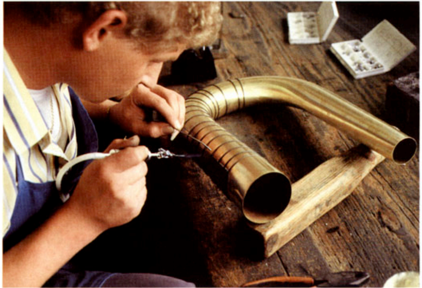
fig.11A. Manufacture and repair of brass type music instruments demands a considerable know-how and feeling for handling the thin sheet metals used to form the air volumes. No wonder that the skilled craftsman demands the ultimate in tools to make his work a perfect masterpiece. Craftsmen appraise the stable, dependable and easily adjustable heat output of the SPIRFLAME ® flame generating system.
