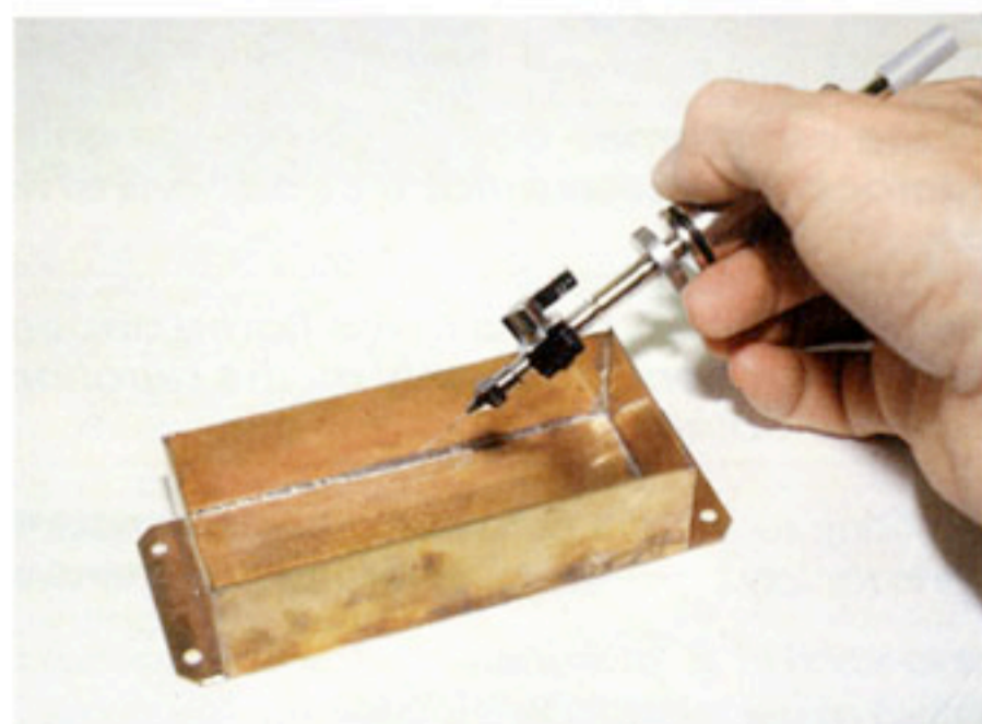
fig.4E. A 2 mm thick copper-bronze alloy sheet is quickly soldered together from several pieces with a minimum amount of heat influx to the assembly.
