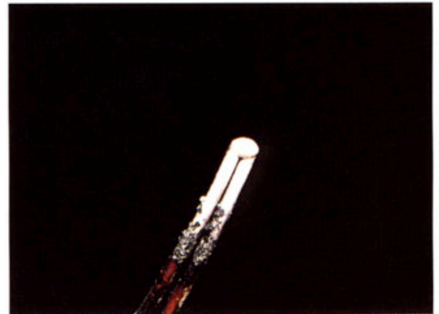
fig.9F. Two magnet wire ends are joined by fusion. The clean, smooth and non-oxidized copper surface indicates a highly reliable weld joint.
