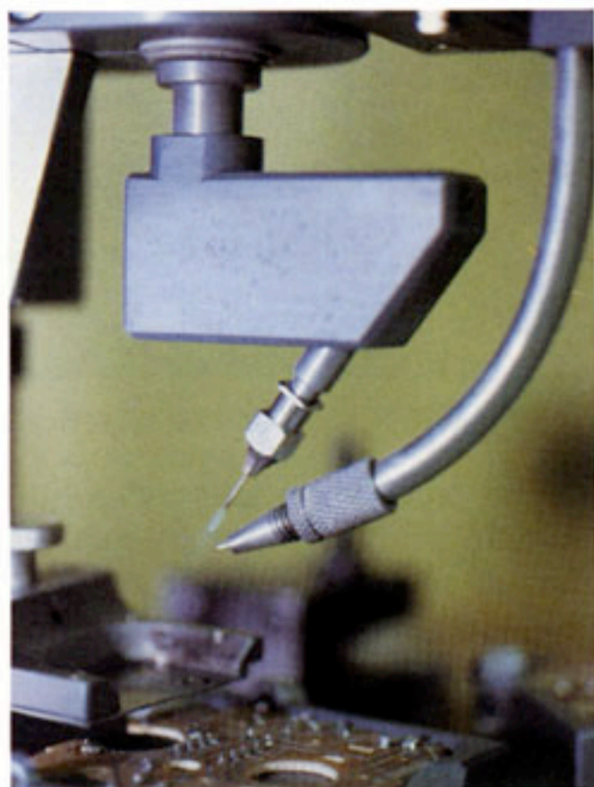
fig.4A. Custom designed "flame handling - solder wire feeder". The relative geometric position of flame and solder wire feed pencil are adjustable. The flame has an almost non-existent side heat radiation and does not heat the nearby solder wire.
