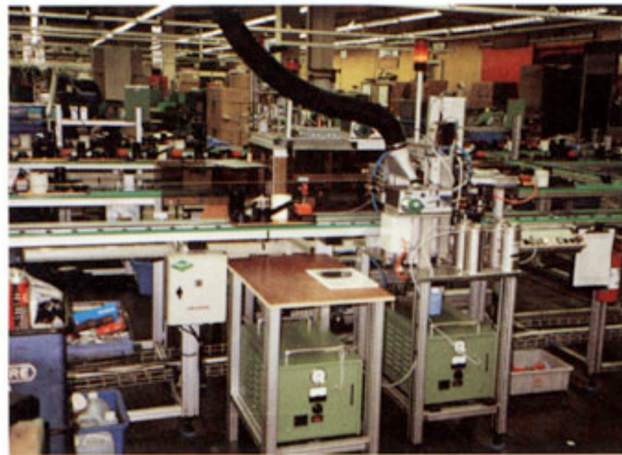
fig.7B. Each of the two SPIRFLAME® units serves one individually adjustable flame in a soft-soldering line for a heater coil installed into a ladies hair dryer. Two simultaneously made joints receive the solder wire from two SPIRIG Solder Wire Feeders LD-200SS . Presence of the two flames is verified by two infrared radiation detectors.
