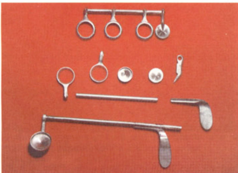
fig.11B / 11C. The low temperature <spirflame> (special additive) does not discolour the polished or lacquer coated metal surfaces during repair of broken instrument parts.
