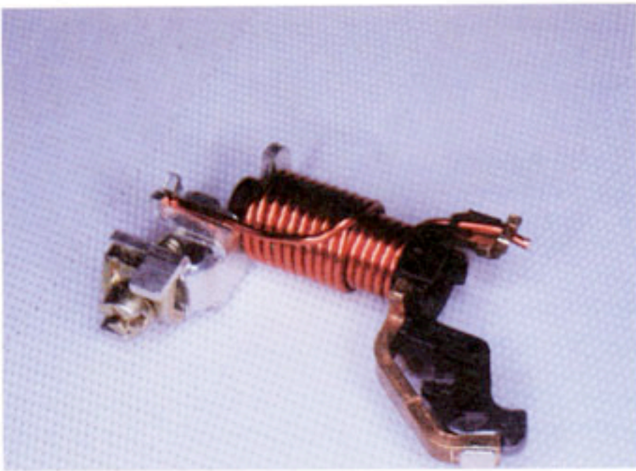
fig.6A / 6B. Assembly of magnetic circuit breakers is made on a fully automated production line. The insulation of the magnet wire is solderable. Both joints are soldered simultaneously with two flames. Each flame is supplied from a separate SPIRFLAME ® to allow maximal flexibility in computer programme controlled flame adjustments.
