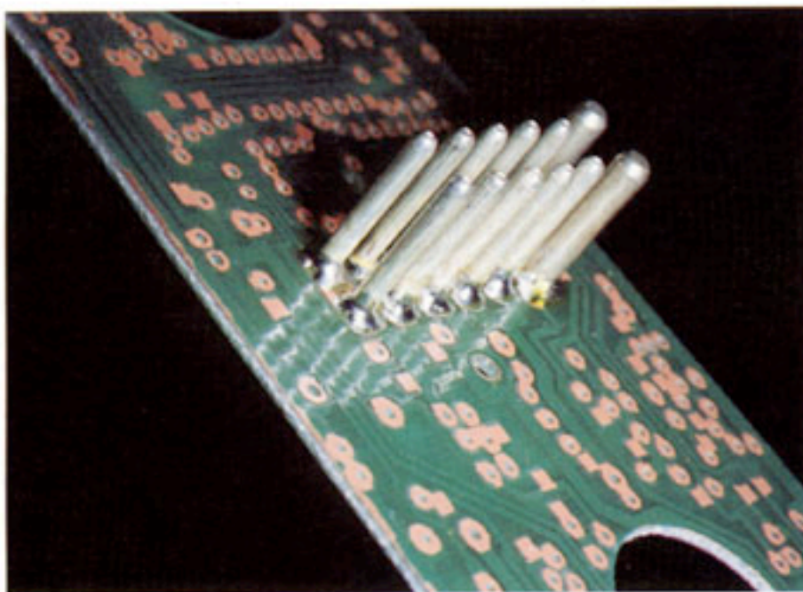
fig.6E. Heavy silver alloy coated connector pins solder directly to this printed circuit board used in automotive electronic systems. The ordinary wave soldering process does not deliver enough heat for a good joint. SPIRFLAME ® eliminates cold solder joints completely.
