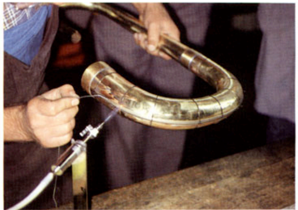
fig.11B / 11C. The low temperature <spirflame> (special additive) does not discolour the polished or lacquer coated metal surfaces during repair of broken instrument parts.
