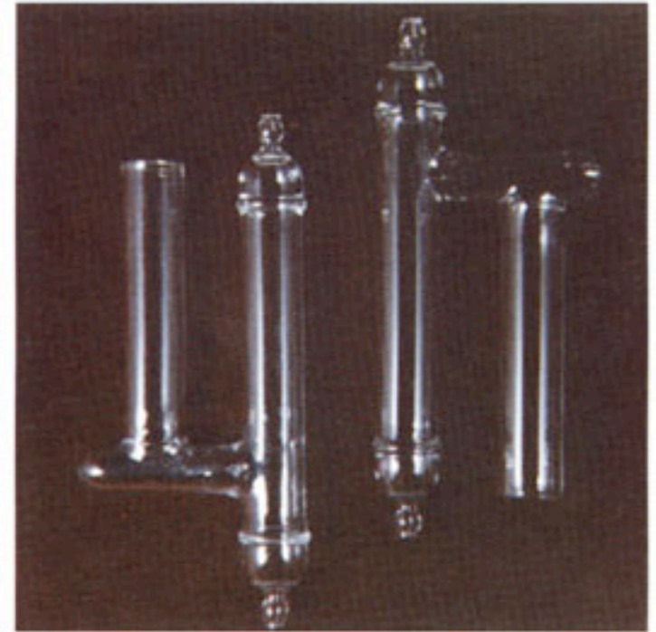
fig.13B. Delicate work on laboratory glass parts and assemblies becomes an easier task with a defined flame heat zone.
