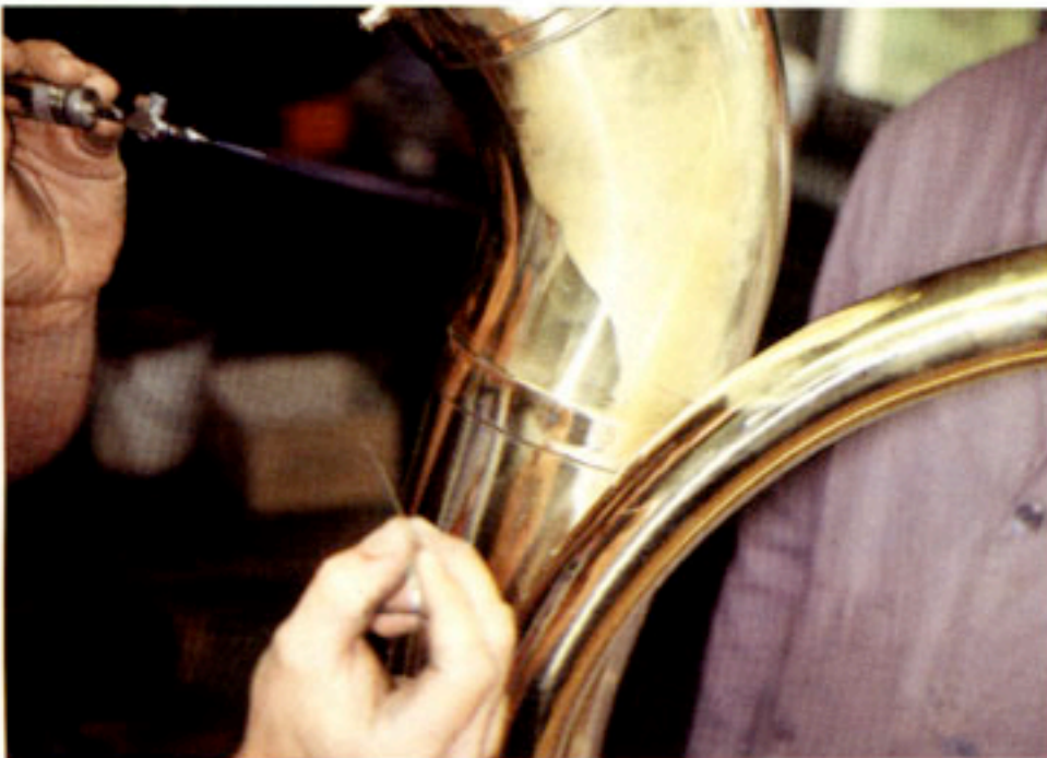
fig.11A. Manufacture and repair of brass type music instruments demands a considerable know-how and feeling for handling the thin sheet metals used to form the air volumes. No wonder that the skilled craftsman demands the ultimate in tools to make his work a perfect masterpiece. Craftsmen appraise the stable, dependable and easily adjustable heat output of the SPIRFLAME ® flame generating system.
